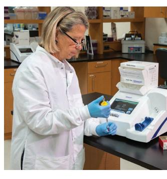
There are many methods for measuring concentration of solutions including: specific gravity, refractive index, and conductivity. Freezing point osmolality, however, is the only method which is truly independent from the size, shape, and other physical characteristics of the liquid solution. This is why freezing point depression is the industrypreferred solution and the gold standard in clinical laboratories around the world.
