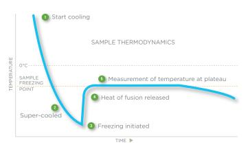
the solution is lowered compared to that of the solvent alone. As more solute is added, the freezing point decreases further. Therefore, by precisely measuring the freezing point of the solution, the osmolality (i.e. concentration) can be determined. Freezing point osmometry can ascertain volatiles in solutions such as CO<sub>2</sub>, ammonia, and alcohol unlike vapor pressure osmometry.
